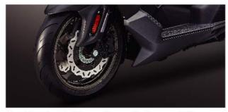
Dual Radial 4-Piston Front Caliper + 275mm Wave Discs with Continental ABS
